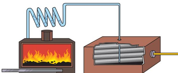
The steam travels under high pressure, through pipes to a big turbine. The high pressure steam is used to spin the turbine.
